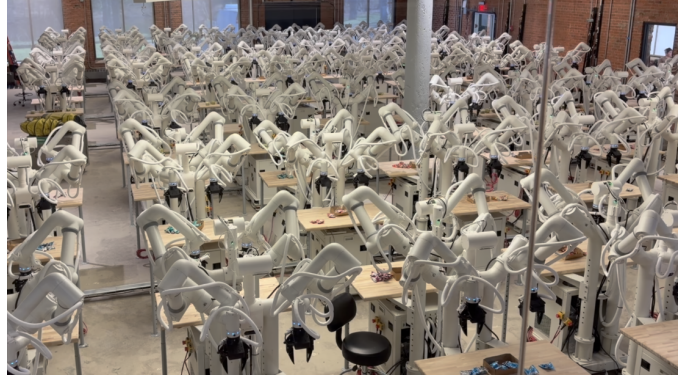
Fig. 1. Data Factory 1 (DF1) . A 100-robot fleet of Sonny bimanual manipulators at Tutor Intelligence HQ in Watertown, MA, collecting up to 1,000 hours of teleoperated demonstrations per day.
